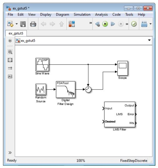
**4** Set the LMS Filter block parameters to model the output of the Digital Filter Design block. Open its dialog box by double-clicking the block. Set the block parameters as follows:
